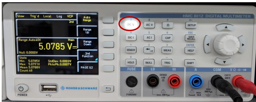
Figure 2. Image of the multimeter showing the configuration to measure voltage.
